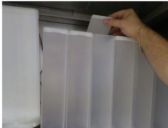
Fig.6.4 - Filling the product containers
