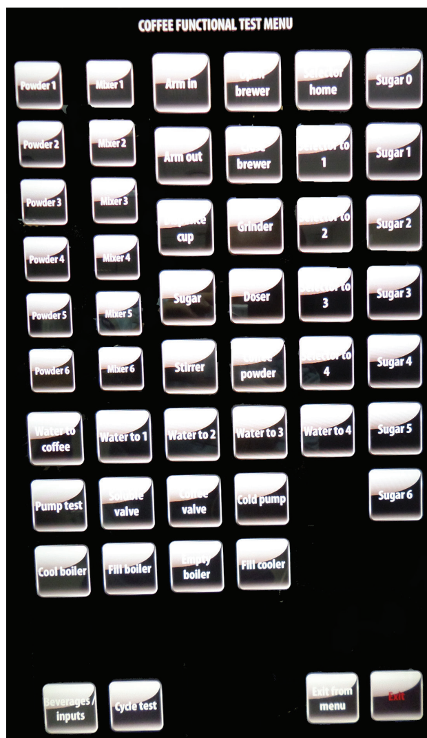
Fig.8.8 - Coffee functional test
